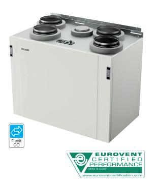
Flexit Nordic S7 SW features patented rotating heat exchanger technology and the Stage Wheel, providing the most energy-efficient ventilation unit on the market with up to 90% thermal efficiency. Low energy consumption and local demand control earn it an A+ eco-design label. Designed for residences and small commercial buildings in Nordic climates, it operates up to 700 m<sup>3</sup>/h and is ideal for residences up to 450 m<sup>2</sup>.
